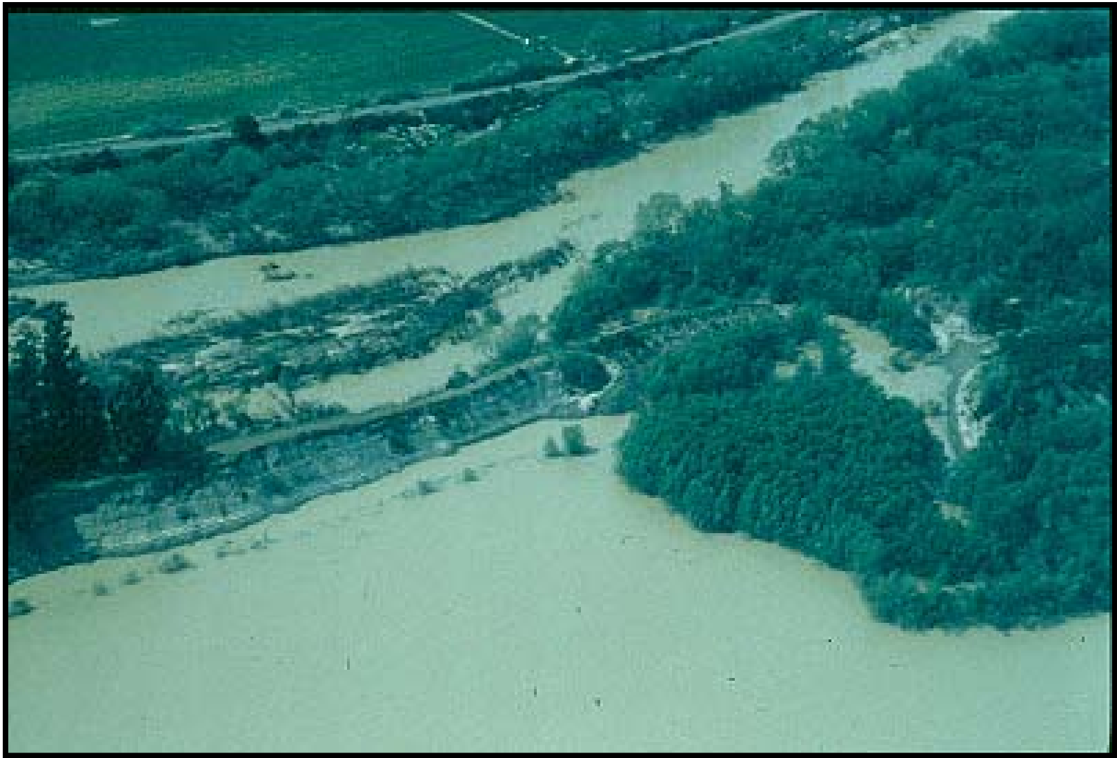
River is eroding the alluvium between the river channel and the pit
