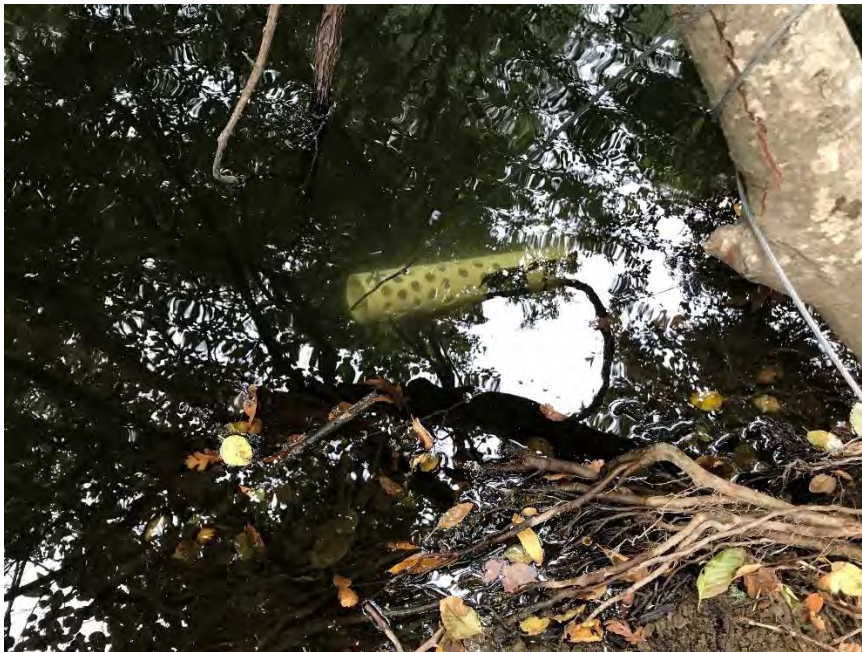
Figure 4. YSI sonde in creek measures water temperature, pH, dissolved oxygen, specific conductance and depth.
