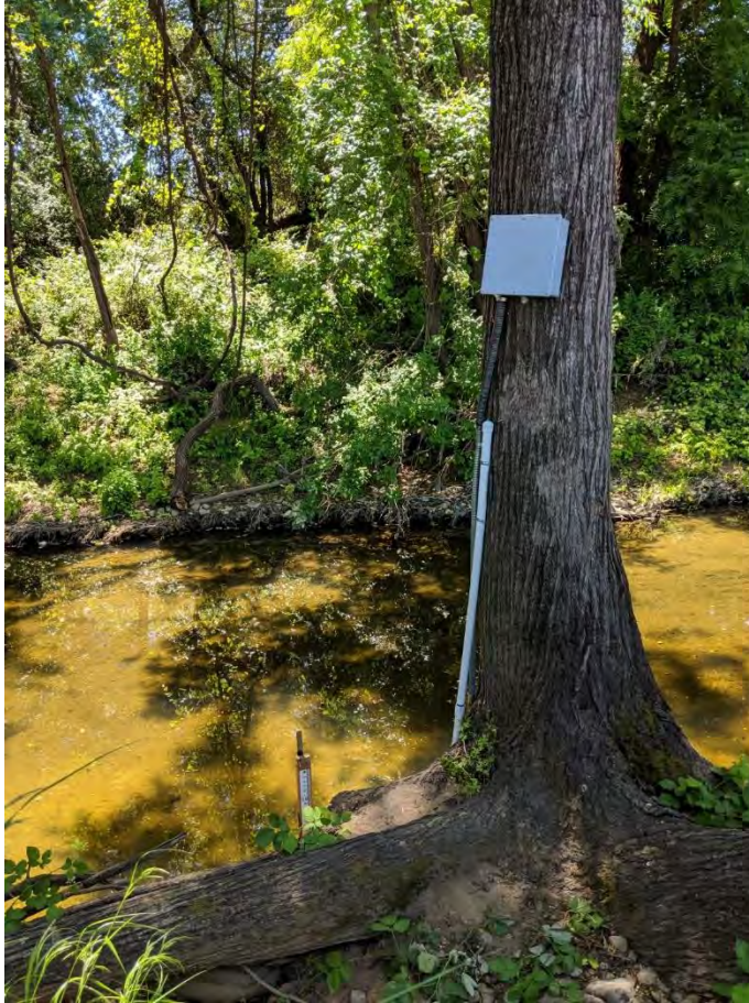
Figure 3. Stream flow gage with pressure transducer and outside staff gage
